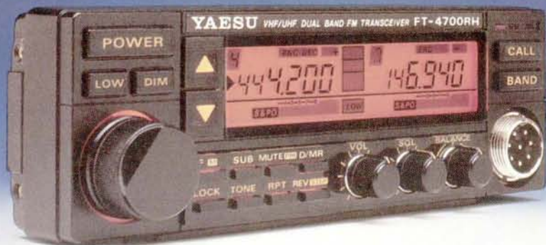
FT-4700RH control head (1 15 / 16 " x 5 7 / 8 " x 1")
